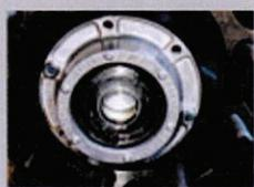
Install the hub cap and torque the bolts refer to torque specification.
